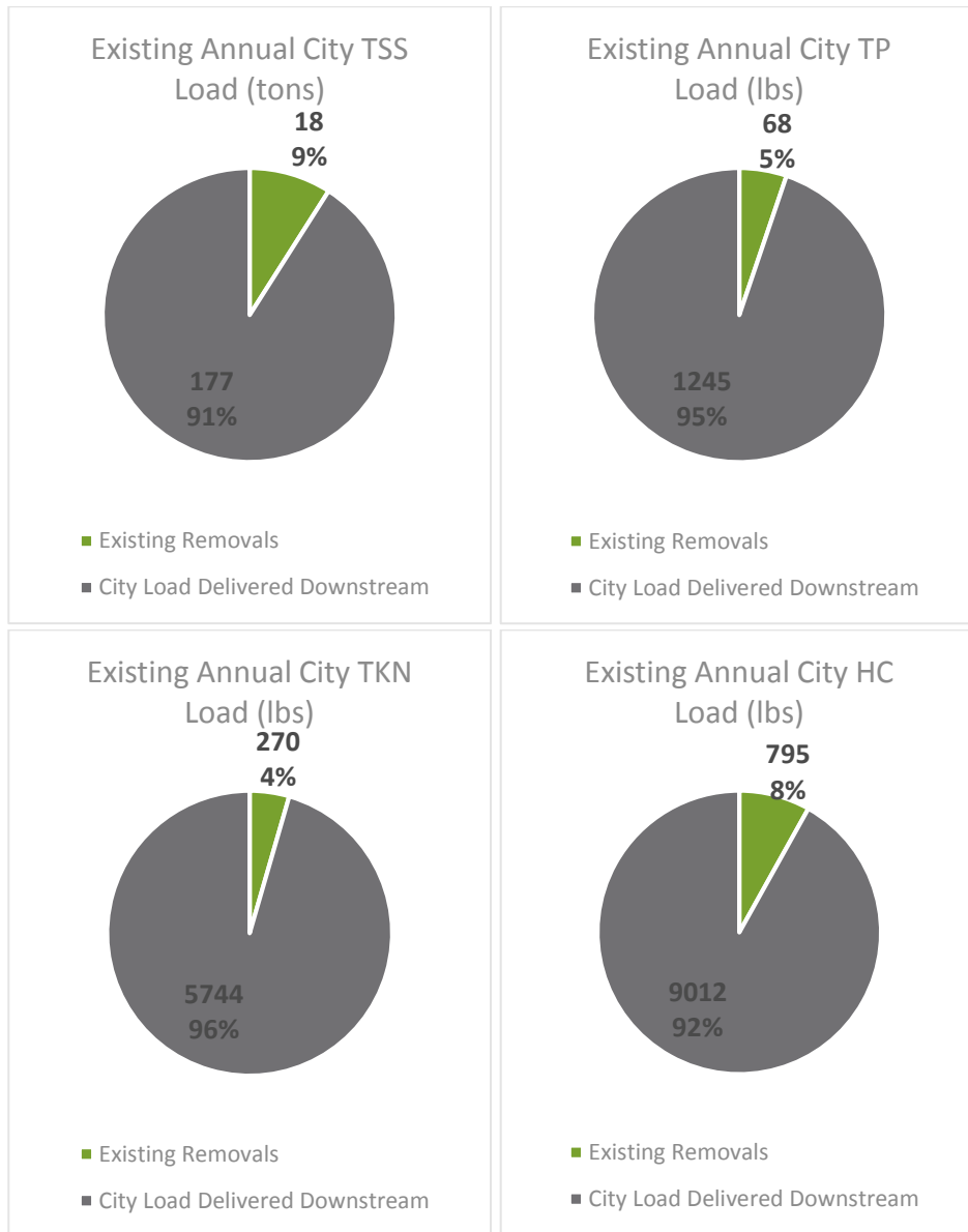
Figure 2: Annual average pollutant removals and delivered loads from within the existing city boundary
